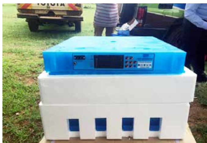
Solar powered egg incubator. Photo: RPLRP, Kenya.
